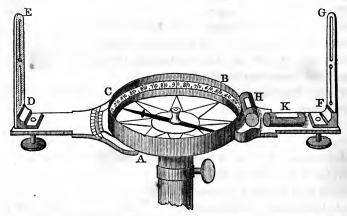
to the plane of the graduated circle, and in each of these there is a large and small aperture for convenience of observation The instrument, when used, is mounted on a tripod, or a single staff pointed with iron at the bottom, so that it may be firmly placed in the ground.
