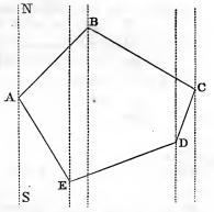
manner with the other sides. If the survey is correct, and the plotting accurately performed, the end of the last side, EA, will fall on A, the place of beginning. This plot is made on a scale of 10 chains to an inch.
