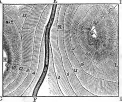
way toward B and L respectively. The angles which the directions GK, GB, GL make with the magnetic meridian being found with the compass, these directions may be represented on paper. Then the measured distances Ga, ab, &c.; Gd, de, &c.; Gg, gh, &c., being set off on those lines of direction, eurves drawn through a, d, g; b, e, h; c, f, k, &c., will show the contour of the hill.
