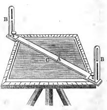
subdivided as minutely as the size of the table will admit. On one side of the board there is usually a diagonal scale of equal parts. A compass box is sometimes attached, which renders the plane table capable of answering the purpose of a surveyor's compass.
