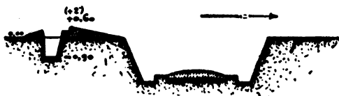
PLATE 27o.—Arrangement for a sunken road defended from the rear.
