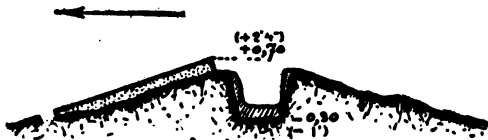
PLATE 27 m.—Arrangement for a dry ditch.
