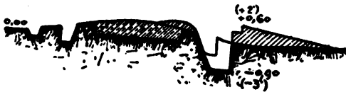
PLATE 27r.—Arrangement of an ordinary road defended on the side toward the enemy.
