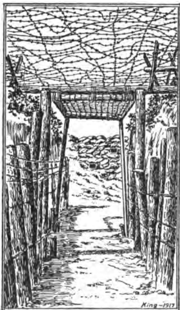
PLATE 45a. —Trench showing wire overhead cover and wire trapdoor obstacle. Machacoulis gallery in background.
