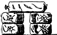
PLATE 22.—Methods of constructing loopholes with sandbags.
