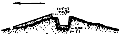
PLATE 27 m.—Arrangement for a dry ditch.
