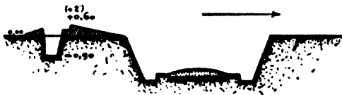
PLATE 27o.—Arrangement for a sunken road defended from the rear.
