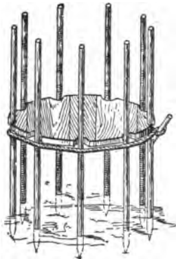
PLATE 36.—Forming the gabion supports.
