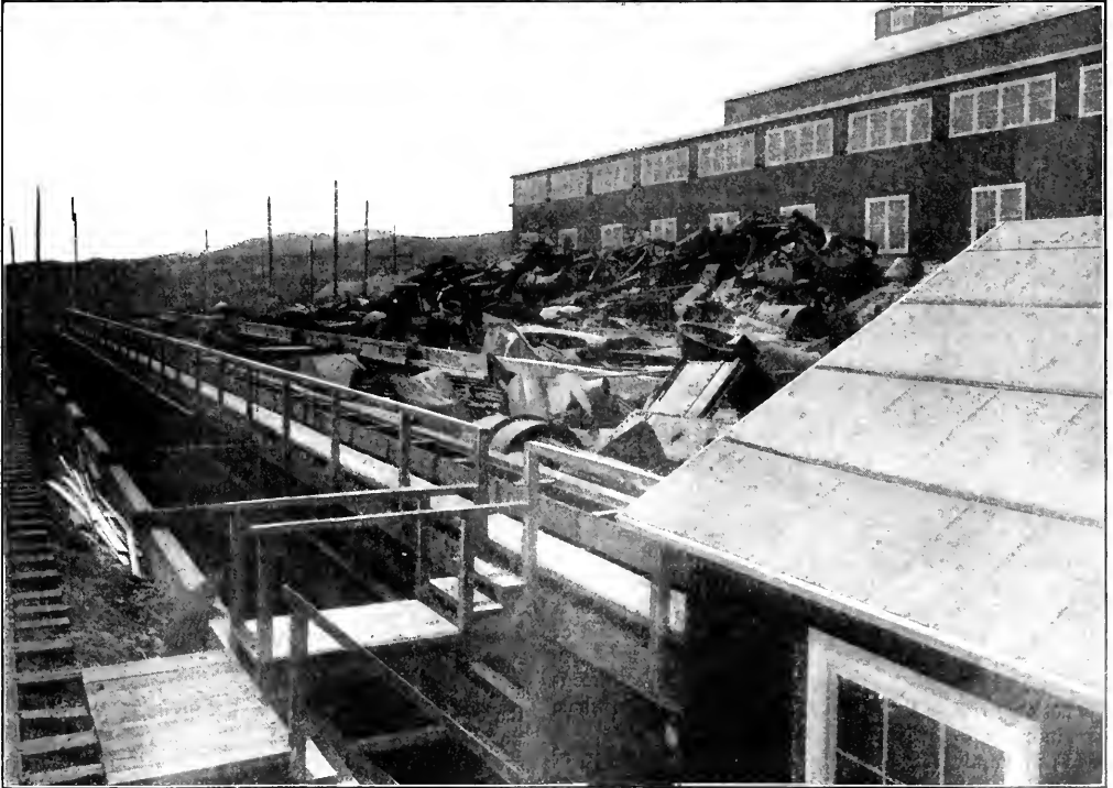
UPPER VIEW—2000-TON LEACHING PLANT OF THE ANACONDA COPPER MINING CO., AT ANACONDA LOWER VIEW—PRECIPITATING TANKS AT THE LEACHING PLANT
