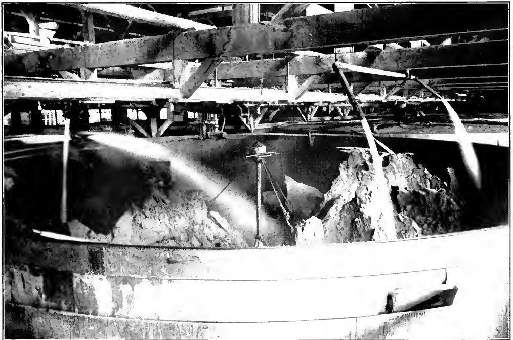
DISCHARGING A SAND TANK BY SLUCING AT THE HOMESTAKE MILL LEAD, S. D.
