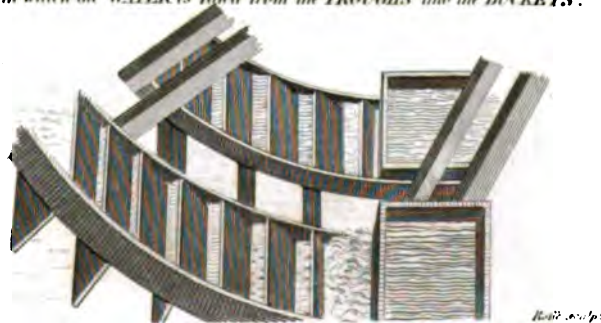
SKETCH of the manner in which the WATER is filled from the TROUGHS into the BUCKETS.
