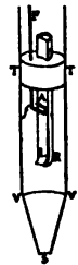
FIG. 2.—Organ pipe fitted with beating reed. AL, Beating reed. R, Reed box. F, Tuning wire. TV, Feed pipe. SV, Conical foot. S, Hole through which compressed air is fed.
