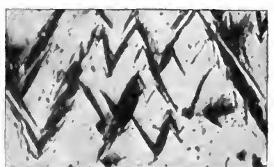
IRON AND STEEL. FIG. 15.—(Osmond.) Martensite (black) in austenite (white). Steel (carbon about 1.5%) quenched at 1050° C. in ice-cold water. Magnified 250 diameters.
