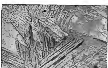
IRON AND STEEL. FIG. 14.—(Osmond & Cartaud.) Martensite. Magnified 250 diameters.
