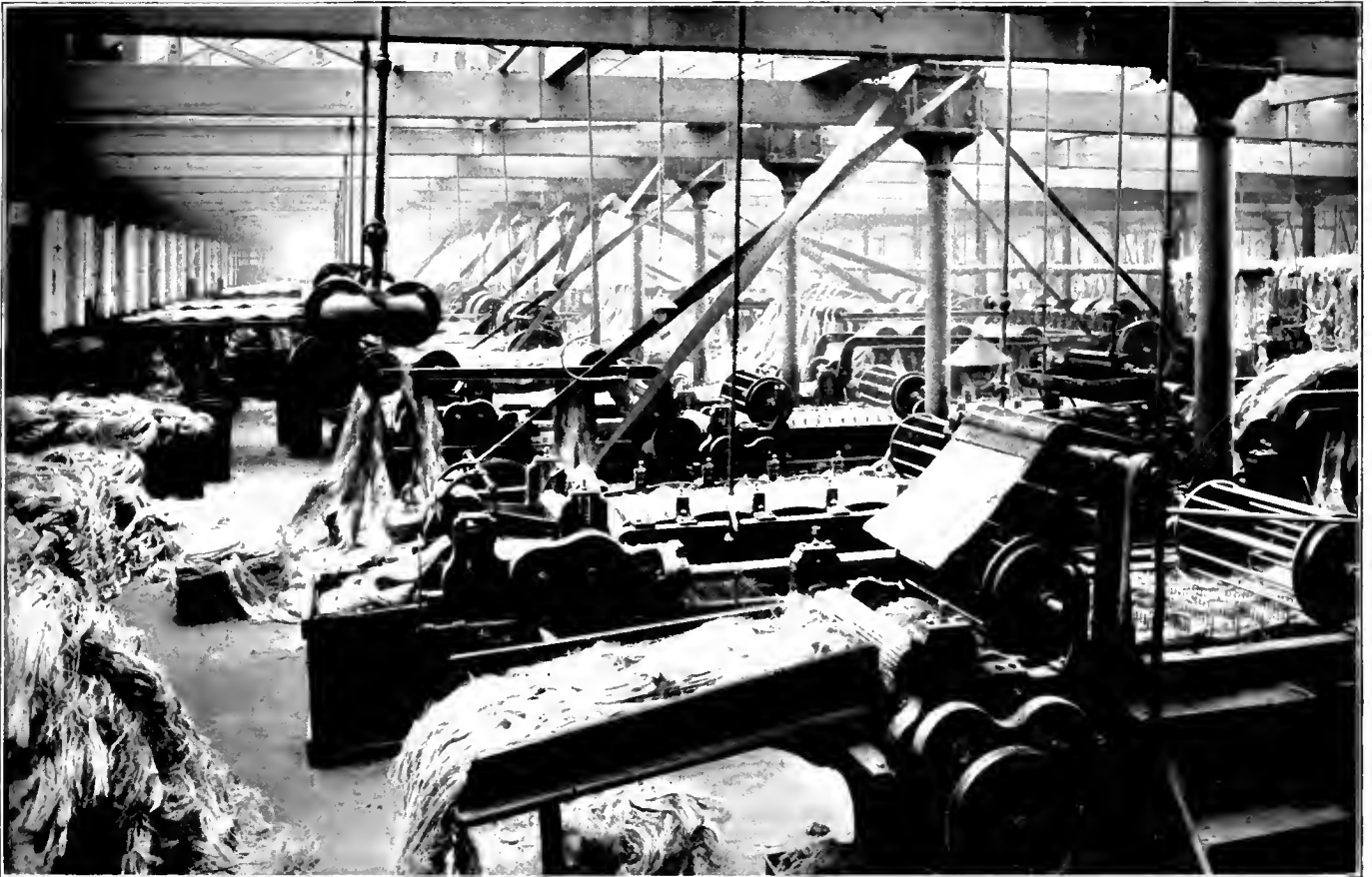
FIG. 10.—MANILA ROPE YARN PREPARING, POTTINGER MILL, OF THE BELFAST ROPEWORK CO. LTD.
