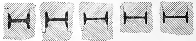
FIG. 8.—Reduction of Girder Section in Finishing Rolls.
