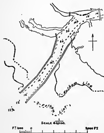
FIG. 9.—Jetty Outlet into Baltic: River Pernau.
