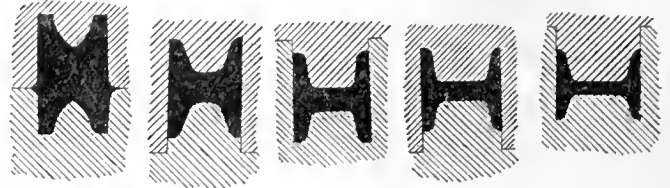
FIG. 7.—Reduction of Girder Section in Roughing Rolls.
