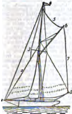
FIG. 7.—Cutter Yacht. 1, bowsprit and martingale; 2, jib—behind it is the foresail; 3, cross-trees and topmast-shroud; 4, pennant designating the club to which she belongs; 5, gaff-topsail; 6, peak of gaff, hoisted by peak and throat halyards; 7, mainsail; 8, end of boom and topping-lift.
