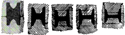
FIG. 7.—Reduction of Girder Section in Roughing Rolls.
