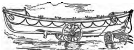
FIG. 1.—The 33-ft., Double-banked, Ten-oared, Self-righting and Self-emptying Life-boat (1881) of the Institution on its Transporting Carriage, ready for launching.
