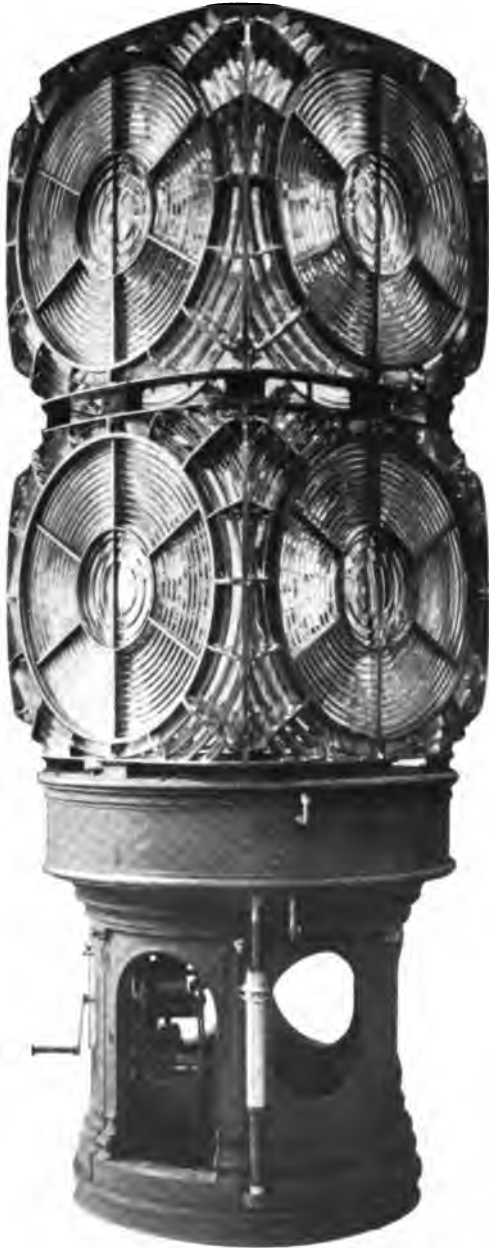
Fig. 54.—Fastnet Lighthouse—First Order Single-Flashing Biform Apparatus.
