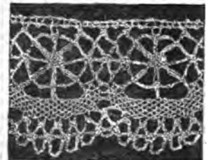
FIG. 58.—Specimen of Machine-made Lace in which the twisting and plaiting of the threads are identical with those of the hand-made specimen of fig. 57. (Nottingham, 20th century.)
