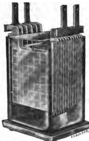
FIG. 25. Manchester-Box Stationary Cell. 1/10 size.
