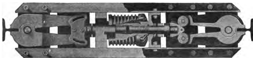
FIG. 13.—Wedge clamp safety.
