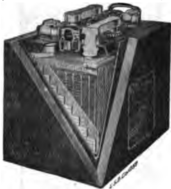
FIG. 26. Three-cell Auto Starting Battery. Approx. 1/6 size.
