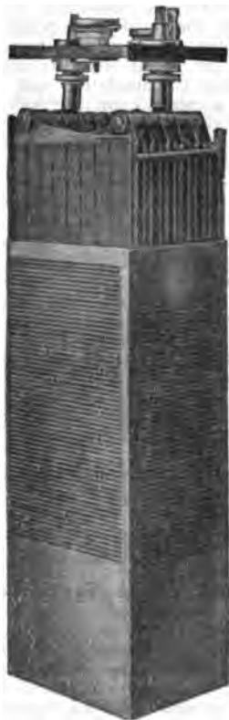
FIG. 4. Edison Cell — for Vehicle and General Service. Plates lifted to show method of assembling. About 1/5 size.
