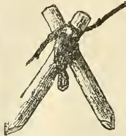
METHOD OF LASHING A PAIR OF SHEERS.
