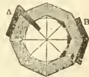
FIG. 78.—Jointing of Column.
