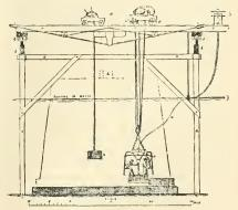
Fig. 3 .- Block-laying by Diving Bell.
