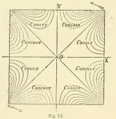
(5.) Diagram of St Venant's curvilineal squares for which torsion problem is adjobraically solvable.—This diagram (fig. 11) shows the series of lines represented by the equation  $x^2+y^2=a(x^4-6x^2y^2+y^4)=1-a$ , with the indicated values for a. It is remarkable that the values a=0.5 and a=0.5
