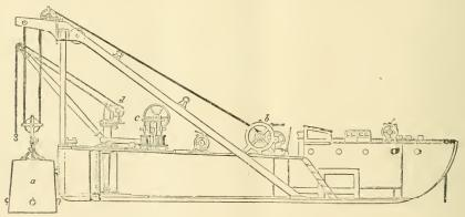
Fig. 4. - Longitudinal Section of Diving Bell Lighter (56 feet long and 21 feet beams,
