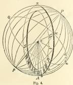
and through the axis Pp draw a plane entting the sphere in 24 equidistant great circles. As the sun revolves round the axis the shadow of the axis will successively fall on these circles at intervals of one hour, and if these circles cross the vertical cited ZMA in the points A, B, C, &c., the shadow of the lower portion Ep of the axis will fall on the lines EA, EB, EC, &c., which will therefore be the required hour lines on the vertical dial, Ep being the style.
