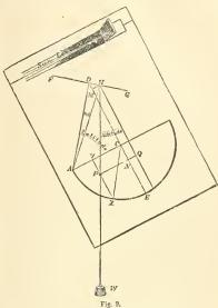
sun-line, or its parallel AC, makes with the horizontal The angle PHQ will be equal to the altitude, if HQ be drawn parallel to DC, for the pair of lines IIQ, HP will be respectively at right angles to the sun-line and the horizontal.
