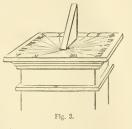
The line of demarcation between the shadow and the light will be better defined than when a wire style is used; but the indications by this double dial will always be one minute too fast in the morning and one minute too slow in the afternoon. This is owing to the magnitude of the
