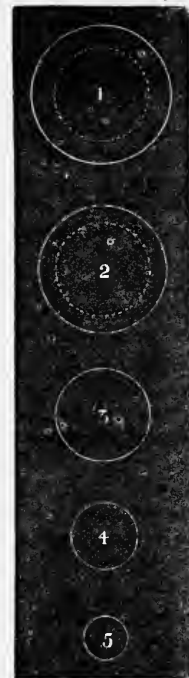
FIG. 16.—Relative Diameters of Back Lenses of Air, Water, and Oil Immersion Objectives.
