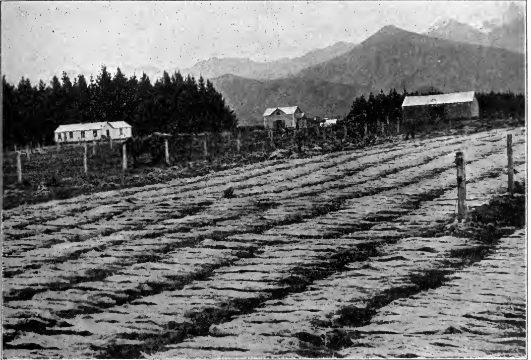
HEMP INDUSTRY Drying Phormium fibre after washing
