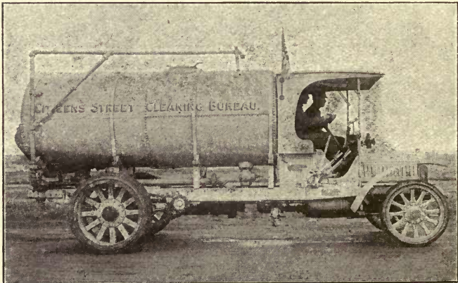
Extension Pipe When Not in Use Folds Over Top of Tank
