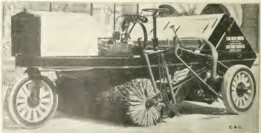
The Elgin Motor Street Sweeper.
