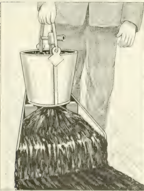
A Hand Bitumen Distributor Delivering Over a Cone Spreader.
