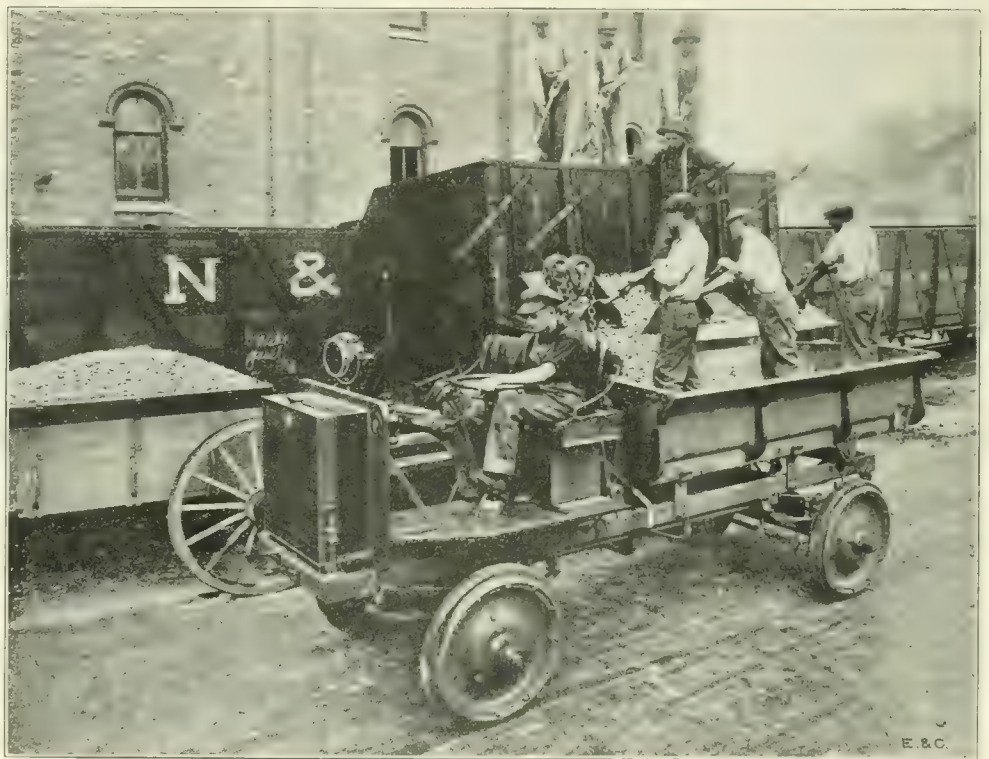
Fig. 1. Method of Loading Motor Truck Used in Hauling Test at Kenosha, Wisconsin.
