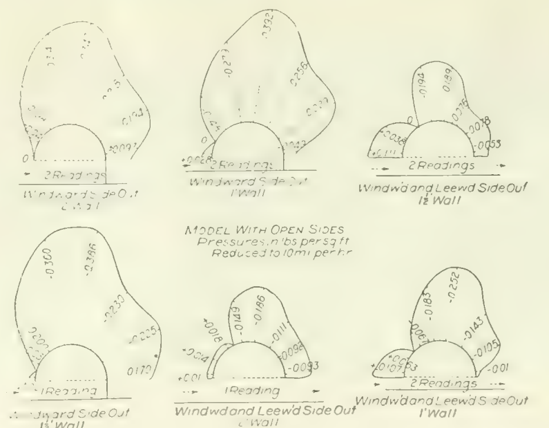
Fig. 3. Pressure and Suction Diagrams for Model Building with One and Both Sides Open.
