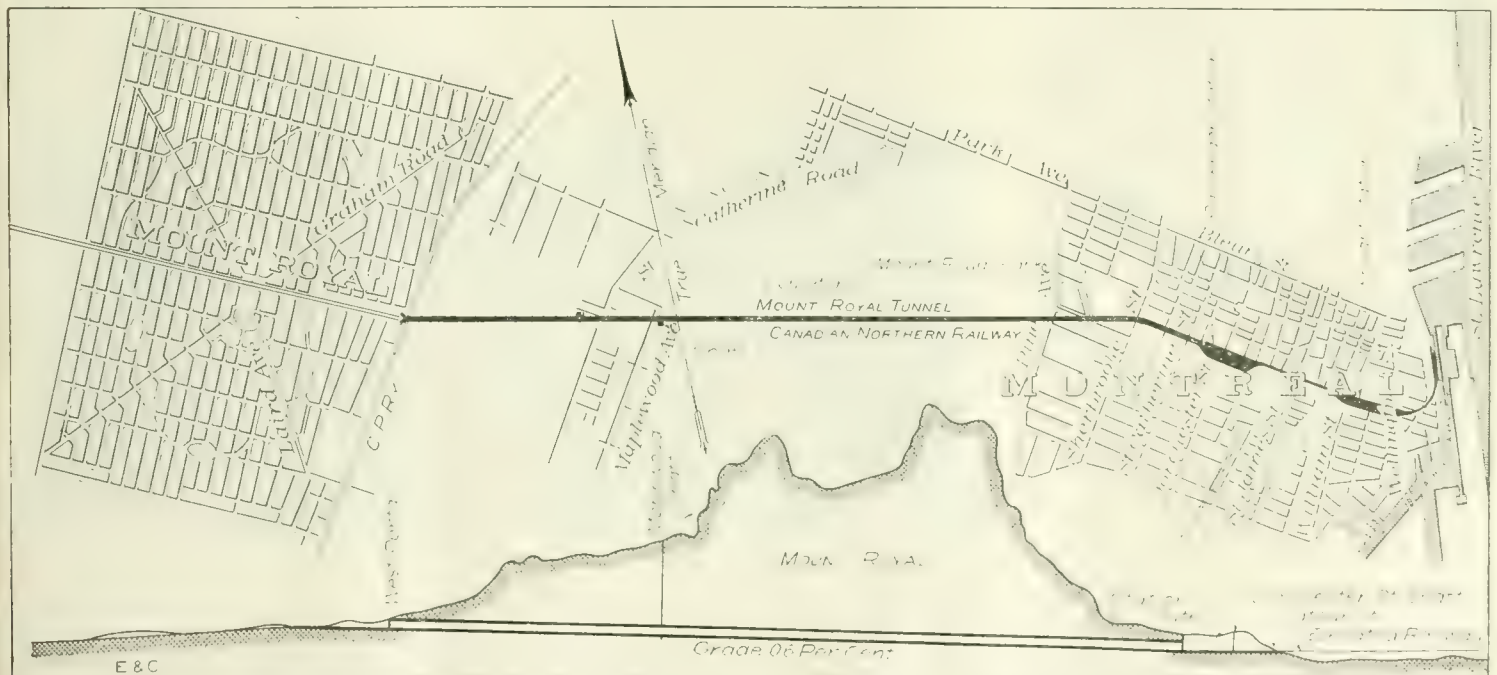
Fig. 1. Plan and Profile of Mount Royal Tunnel, Canadian Northern Ry., Montreal, Can.
