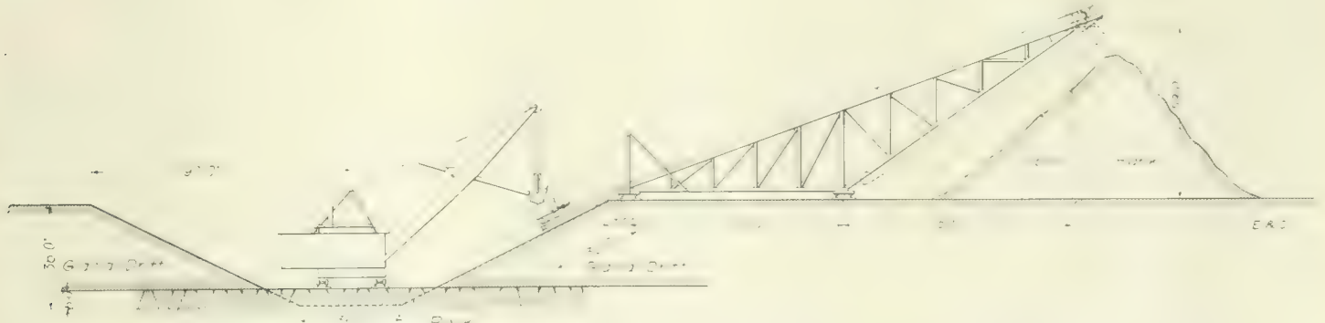
Diagram Showing Arrangement of Revolving Steam Shovel and Steel Tippie for Canal Excavation.
