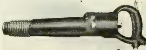
Pneumatic Riveter With Spiral Rivet Set Retainer.
