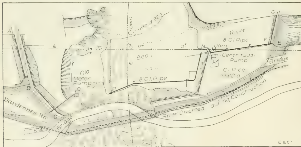
Fig. 10. Plan Showing Works for the Diversion of the River During the Construction of the Dam.
