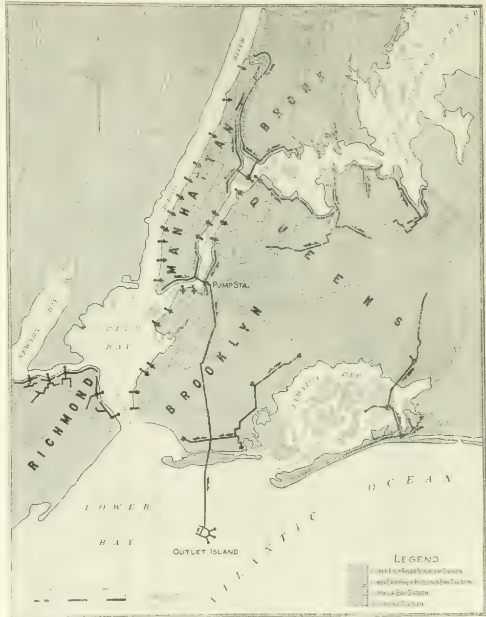
Fig. 1. General Plan Showing Main Drainage and Sewage Disposal Works Proposed for New York City by the Metropolitan Sewerage Commission, 1914.
