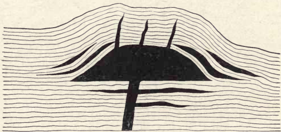
FIG. 52. — Section through laccolith showing associated sheets and dikes. Compare outline of laccolith with that of Fig. 53.
