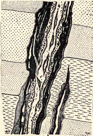
FIG. 212.—Vein filling a fault fissure. Enterprise mine, Rico, Col. (After Rickard, Amer. Inst. Min. Engrs., XXVI, 1897.) Shows irregular banding, also vugs in center of vein. White vein material is quartz; dark, is blende and rhodochrosite.
