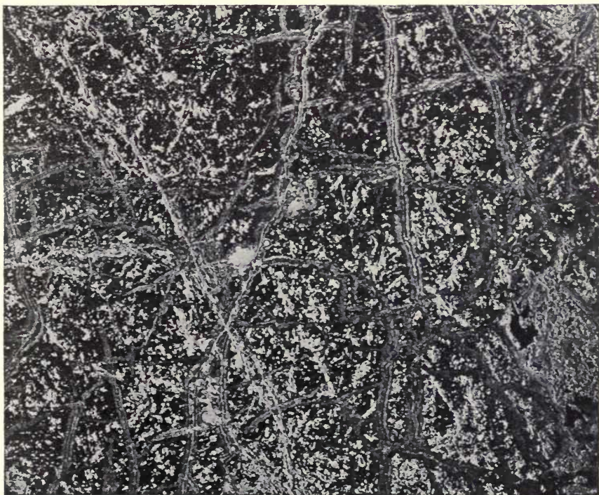
FIG. 3.— Secondary chalcocite in fractures in bornite, \times 10 diameters. The mass of bornite is penetrated in all directions by a network of chalcocite veinlets. All from Virgilina copper district. (After Laney.)
