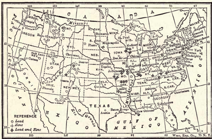
FIG. 225. — Map showing distribution of lead and zinc ores. (After Ransome, Min. Mag. , X.)
