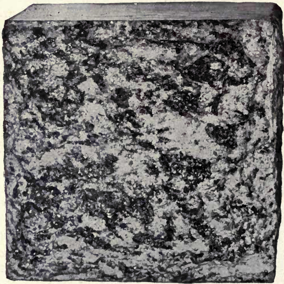
FIG. 2. — Port Deposit, Maryland, gneissic granite with face cut parallel to the banding.
