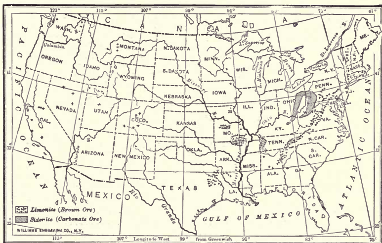
FIG. 224. — Map showing distribution of limonite and siderite in the United States. (After Harder.)
