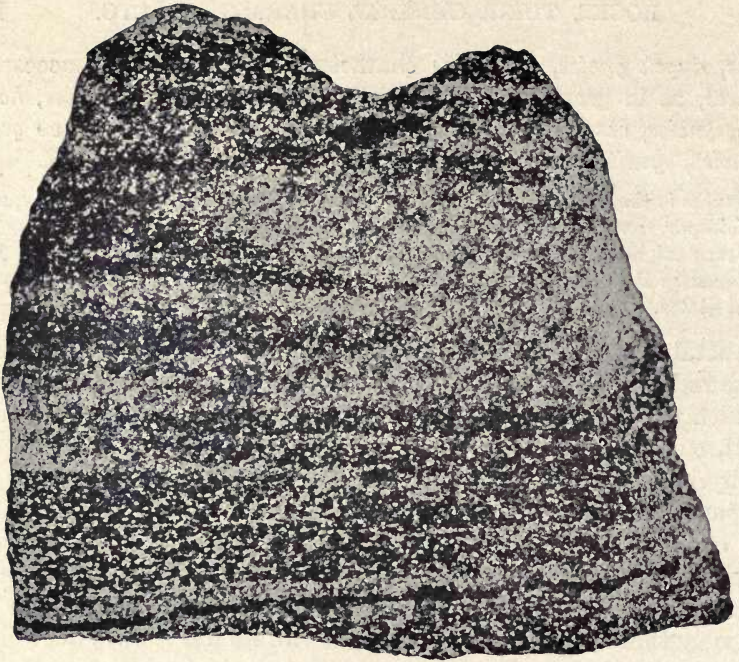
PLATE XVI, FIG. 1. — Hornblende gneiss, showing irregular banding. Dark patches, hornblende; light areas, mixed quartz and feldspar. (From Ries, Building Stones and Clay Products.)
