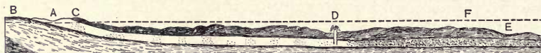
FIG. 154. — Section illustrating the transition of a porous water-bearing bed, A, into a close-textured, impervious one. Being inclosed between the impervious beds, B and C, it furnishes the conditions for an artesian fountain at D. (After Chamberlin.)
