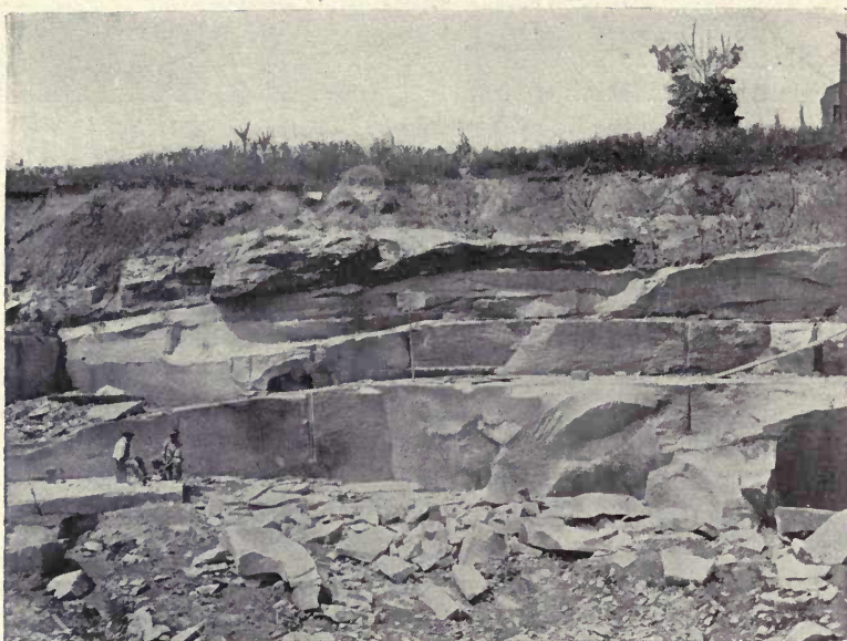
PLATE XXXIV, FIG. 1.—Granite quarry, Manchester, Va. Shows sheeted structure of granite and covering of residual clay. (H. Ries, photo.)
