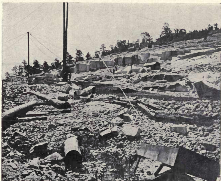
FIG. 2. — Quarry of granite along base of Stone Mountain, Ga., shows sheeting following surface. (After Watson, Ibid. )
