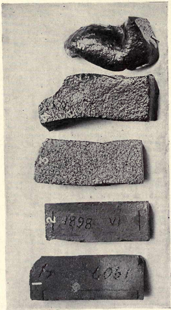
PLATE LXXXVI. — Bricklets of different clays, all fired at the same temperature to show their different fusibilities. (512)
