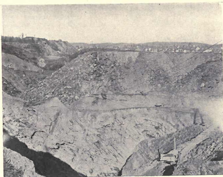
FIG. 2. — Slate quarry, Penryn, Pa., showing folded beds and cleavage. (H. Ries, photo.)
