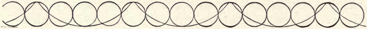
FIG. 172. — Series of particles in their orbits. The circles represent the orbits of the particles which revolve from left to right. At any given moment each particle is advanced in its orbit 90 degrees more than its neighbor to the right. The curved line representing the form of the wave, advancing from left to right, connects the simultaneous position of all particles.
