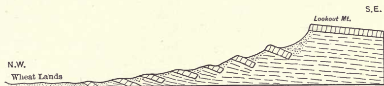
FIG. 170.—Ideal profile of landslides on the northern side of Lookout Mountain, Wash. (After Russell, U. S. Geol. Survey, 20th Ann. Rept., Pt. II.)
