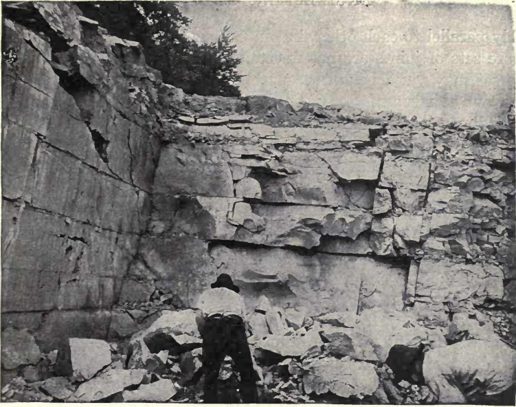
PLATE XXII, FIG. 1. — Limestone showing horizontal bedding, and one set of vertical joints. The flat face of the quarry is a joint surface of a second set. Cement rock quarry, Milwaukee, Wis. (H. Ries, photo.)
