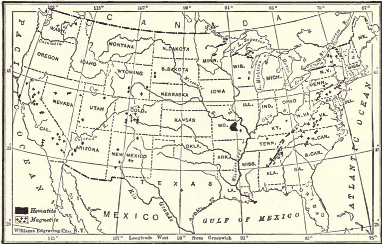
FIG. 223. — Map showing distribution of hematite and magnetite in the United States. (After Harder, U. S. Geol. Survey, Min. Res., 1907.)
