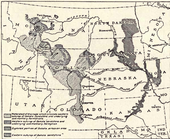
FIG. 165. — Darton's map of catchment area of the Dakota sandstone and the Dakota artesian basin. (After Slichter, U. S. Geol. Survey, Water Supply Paper, 67.)
