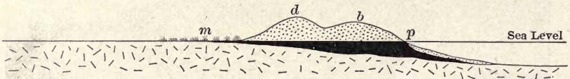
FIG. 183. — Section of a barrier beach which has moved inland, part way across a marshy lagoon. b , barrier; m , marsh; p , peat; d , dune. (After Goldthwait, Ill. Geol. Survey, Bull. 7, 1908.)
