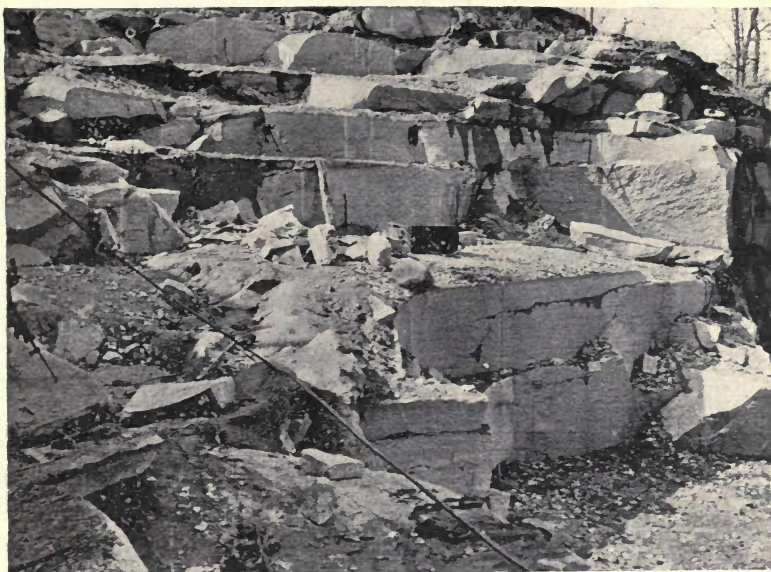
PLATE XXIX, FIG. 1. — Granite quarry, near Woodstock, Md., showing horizontal joints. (T. L. Watson, photo.)
