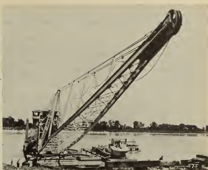
Fig. 4—Dredge boat equipped with a boom 240 ft. in length. A boom of this unusual length is made possible by the use of aluminum alloys in the outer 150 ft. of the length
