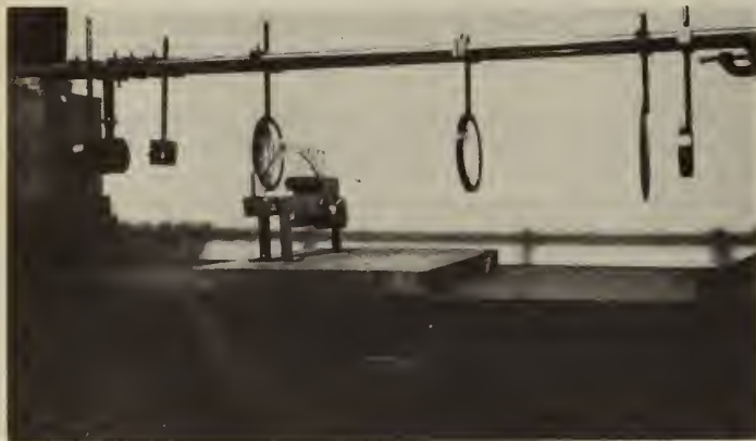
Fig. 1—The Polariscopes, from left to right—lamp housing, polarizer, plano-convex lens, quarter-wave plate, plano-convex lens set so that rays strike model normally, another similar lens, quarter-wave plate, and analyzer
