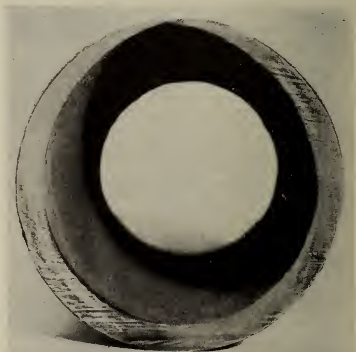
Fig. 1 —Section of heavy walled tube which has been overheated, bulged and split
