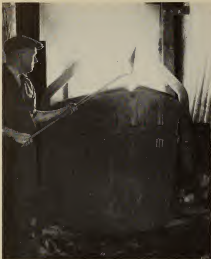
Fig. 5—A stream of molten nickel pouring into the huge waiting ladle as one of the furnaces is tapped in the refinery at Port Colborne
