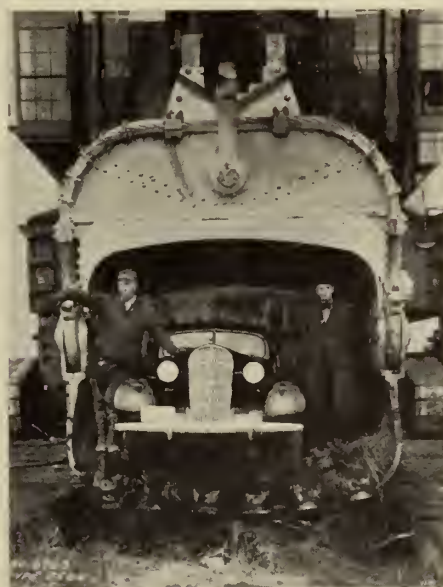
Fig. 5—A 32 cubic yard power shovel dipper built largely of aluminum alloys
