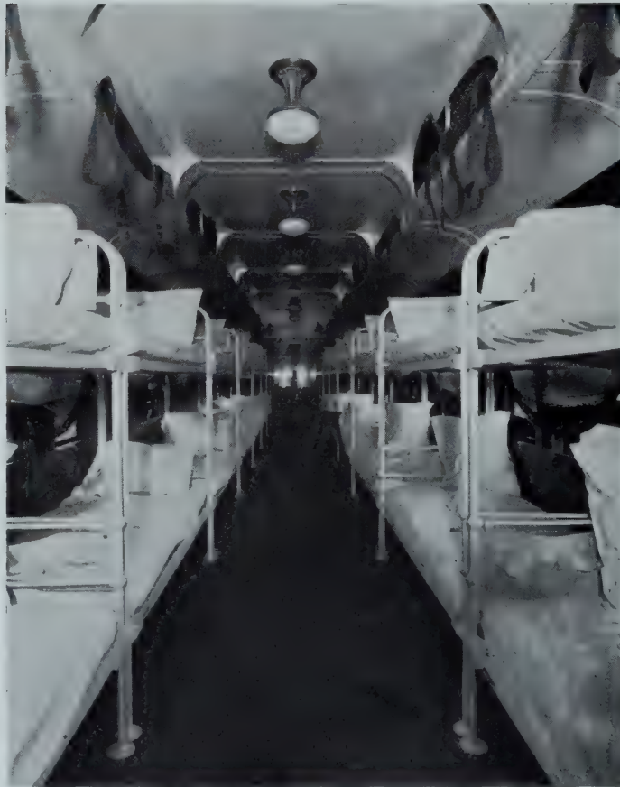
The latest type of hospital car in service on Canadian railways can accommodate twenty-eight bed cases.
