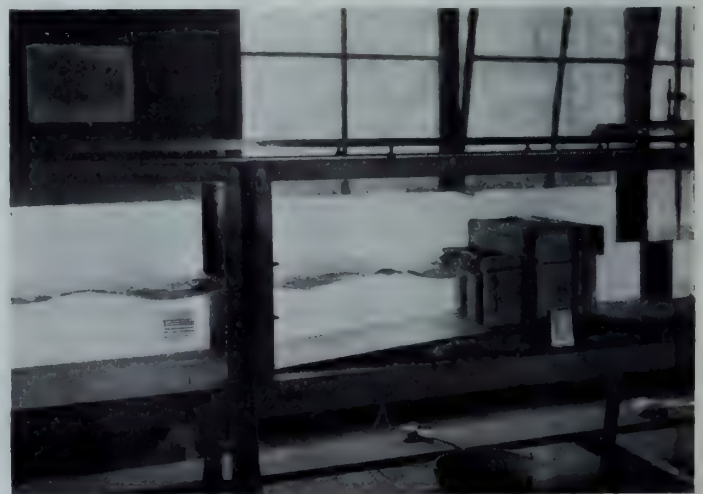
Fig. 17—Surge in tailwater accompanying unstable flow condition in original model of Port Dalhousie outlet works.
