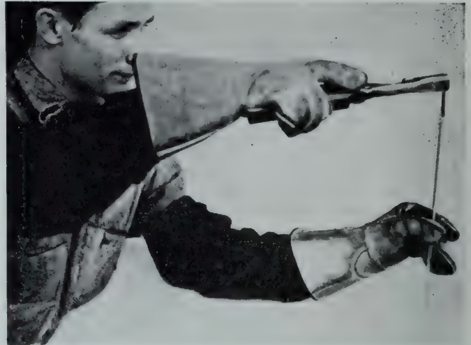
Fig. 2—Illustrating the joining of full fluxed electrode to separate stub.
