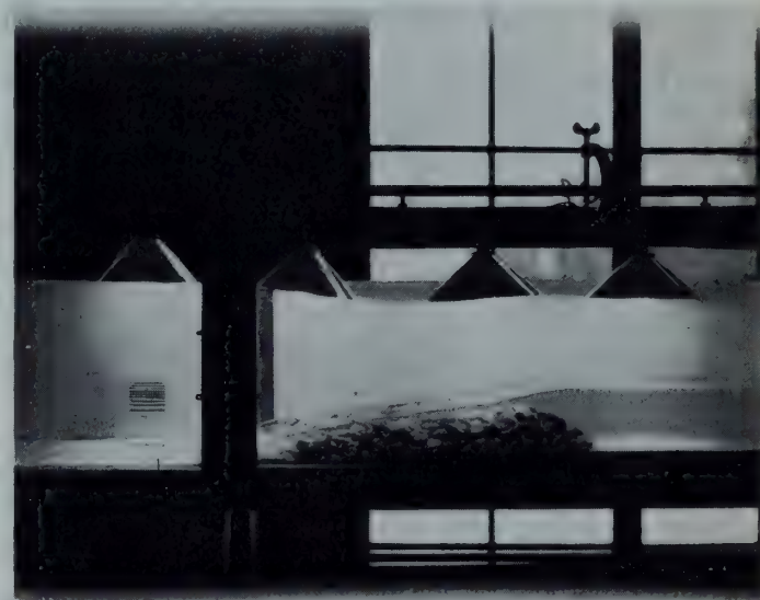
Fig. 13—Model of rock-fill tailrace weir discharging maximum flow at minimum tailwater level, (most severe conditions for stability).
