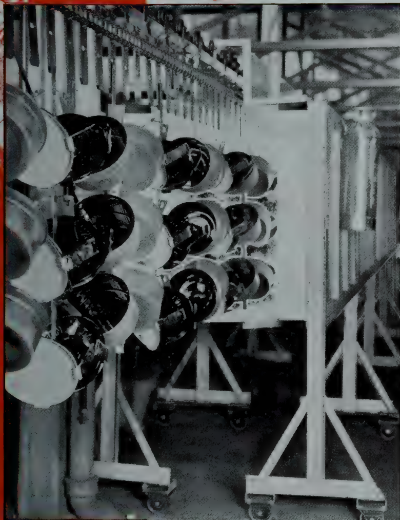
Curing a number of finishes on land mines in one operation.
