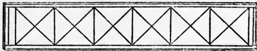
FIG. 20.—This is a "Lattice Girder." The flanges are built up of plates and angles, as in a plate girder, but instead of the solid-plate web, there is a system of struts and ties.
