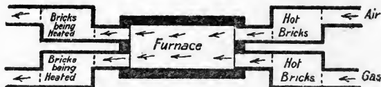
FIG. 16.—Diagram showing how the waste gases in a Regenerative Furnace are made to give up some of their heat, which later is carried back into the furnace.
