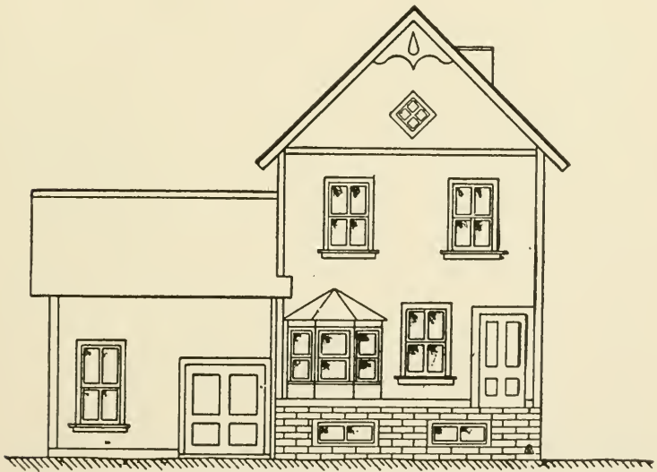
FIG. 4.— FRONT ELEVATION OF A TYPICAL SUB-STATION.
