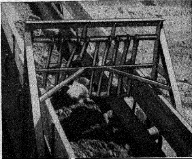
FIG. 17. Swinging steel bars arranged to prevent rollback of lumps on an inclined conveyor. Bars placed at intervals along the belt swing freely in the direction of belt travel but cannot swing backward beyond their normal at-rest position.
