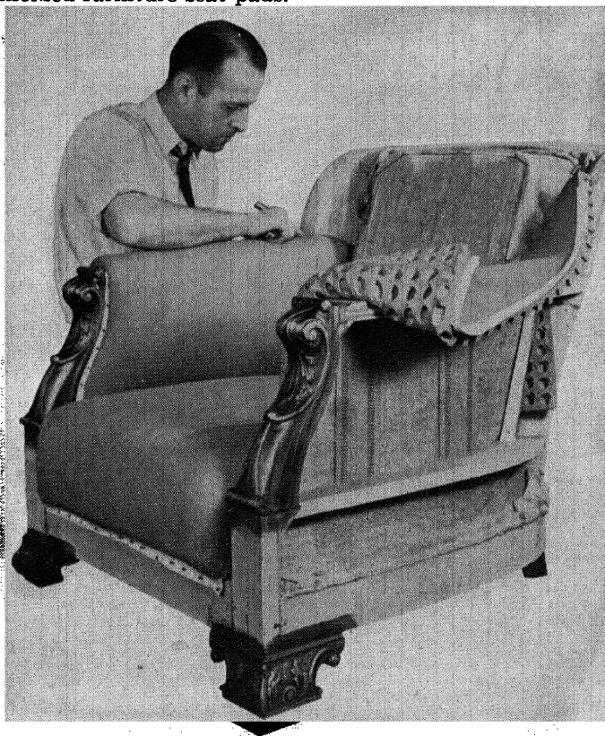
FIG. 2. Upholstering a chair in which latex foam, a form of sponge rubber, is the cushioning material. The rubber cushioning elements may be either molded to shape or made from flat slabs that are easily shaped as desired.
