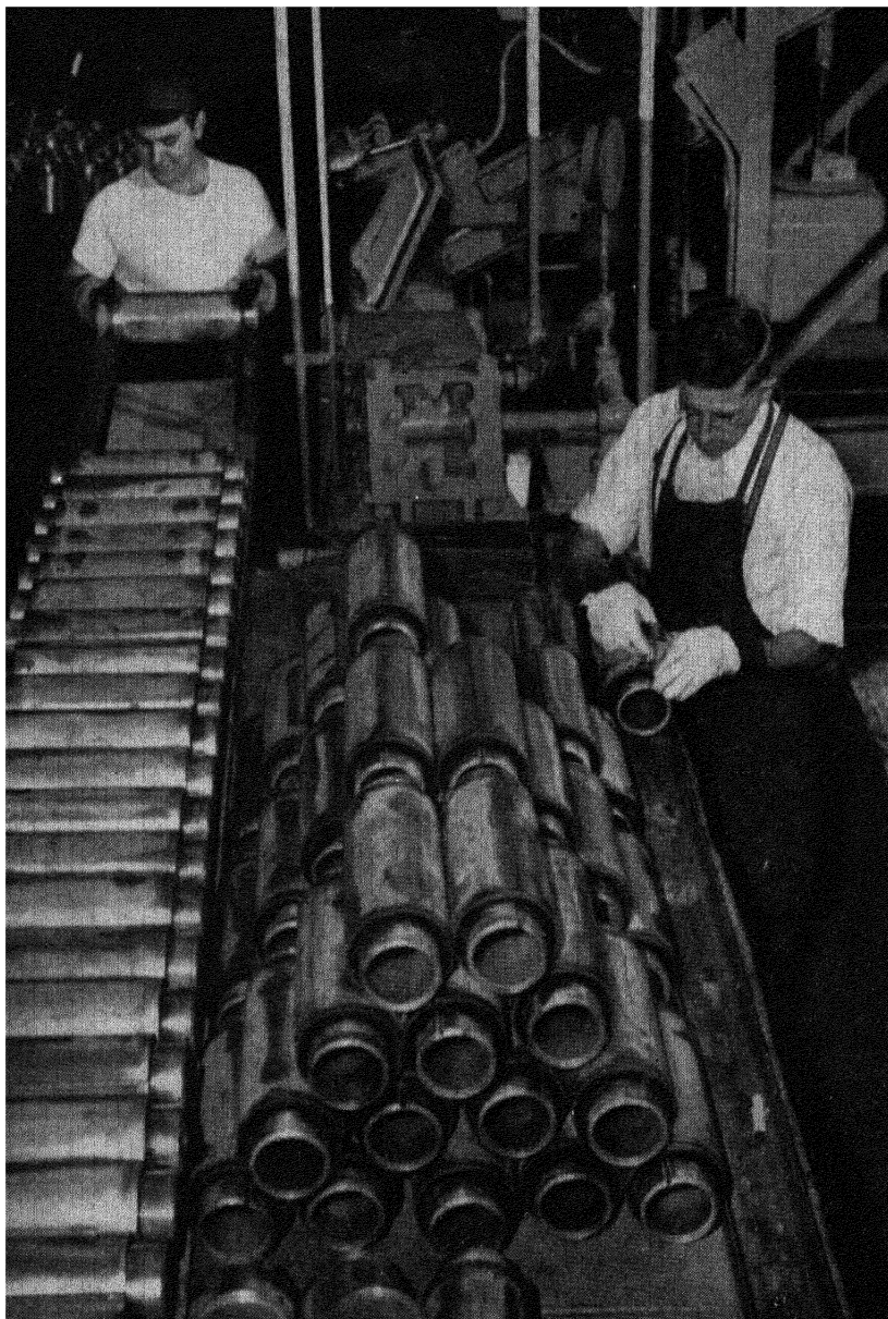
FRONTISPIECE. Typical of rubber's diversified industrial application is this Torsilastic rubber spring, which can be engineered to serve as the suspension member for thousands of industrial, commercial, and automotive uses including stationary motors, industrial trucks, office chairs, railroad coaches, passenger cars, trucks, busses, airplane landing gear, farm implements, drilling equipment, seats of all types, door hinges and springs, streetcars, motorcycles, physical-exercising equipment, truck tail gates, wagons, bicycles, and even built-in ironing boards and rocking chairs.
