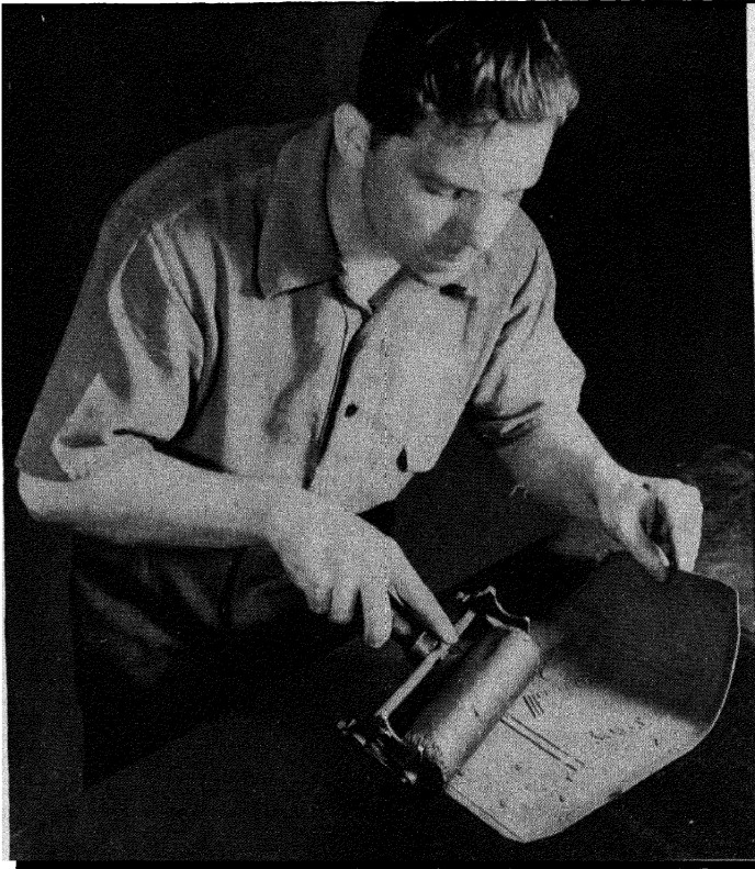
FIG. 7. Rolling a vulcanized rubber printing plate into contact with a base fabric preparatory to placing the plate on a printing press.
