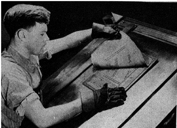
FIG. 4. Removing a molded-rubber printing plate from the resin matrix against which it was vulcanized.
