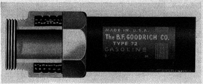
FIG. 11. Gasoline-pump hose showing a coupling attached by expanding a bronze sleeve into the hose wall. Internal ridges of the coupling grip the hose cover.
