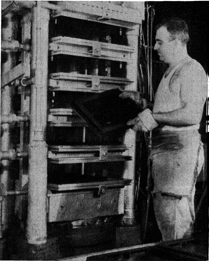
FIG. 3. This multiple-deck vulcanizing press handles five molds at once.
