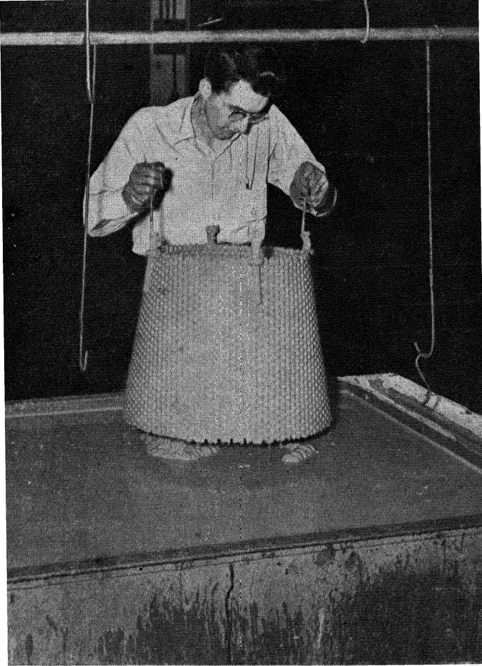
FIG. 4. Draining excessive latex from perforated metal screen. Next step is to vulcanize the coating.
