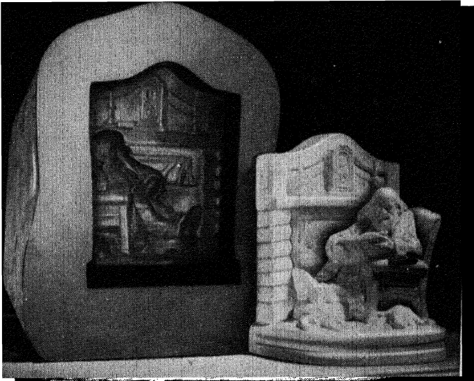
FIG. 11. A plaster book end having undercut details, and the Koroseal mold in which it was produced.
