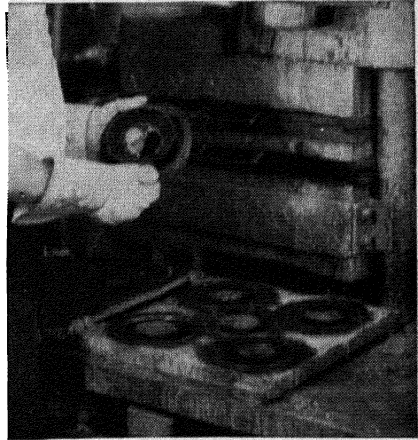
FIG. 6. An accurate, uniform product is assured by proper use of overflow or rind cavities into which excess rubber can flow (see Fig. 5A). The workman is about to tear the rind from a molded ring.
