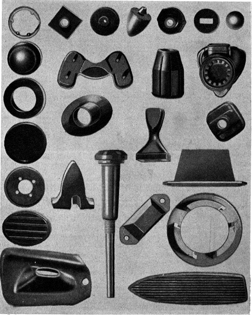
FIG. 1. This collection of rubber parts shows the variety of shapes that can be produced by molding.
