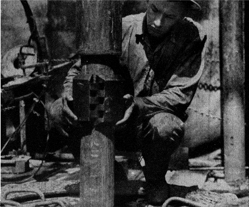
FIG. 8. Fitting a split rubber collar around a pipe used in drilling an oil well.
