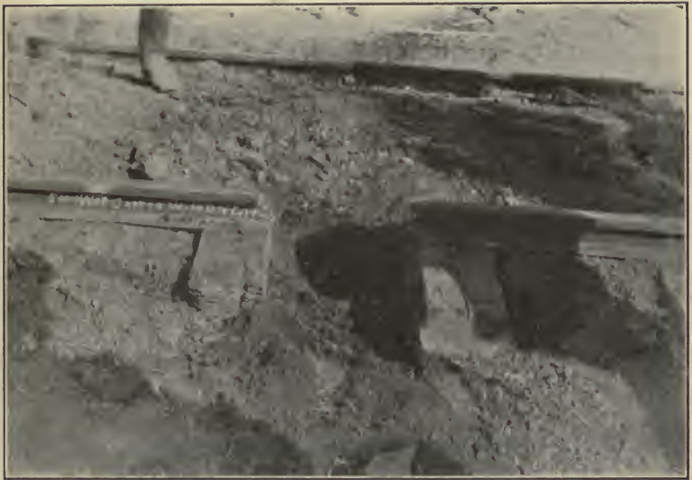
FIG. 55.—Rail cut by 5 oz. of gun-cotton.
