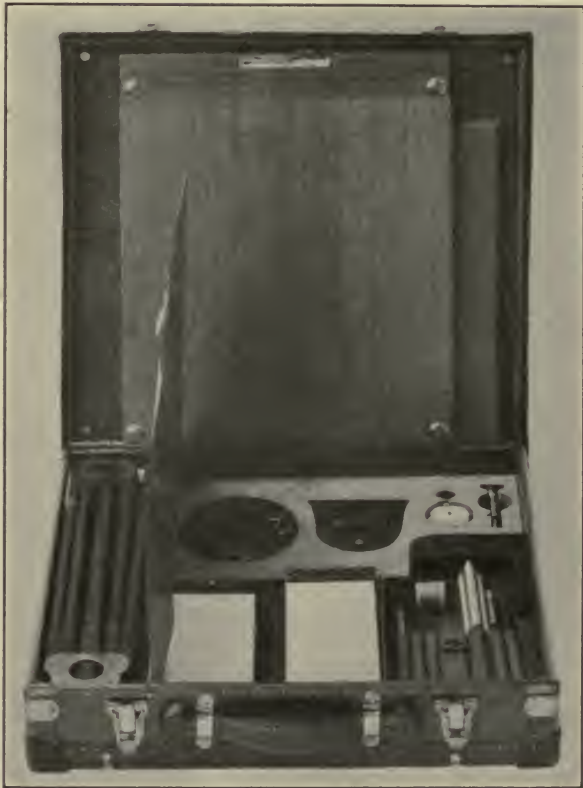
FIG. 62.—Military sketching (mapping) equipment in case. Sketching board with declinator, scales of map distances, slope scale and paper clamps; tripod; prismatic compass; clinometer; stop-watch; alidade; pads, pencils, etc.
