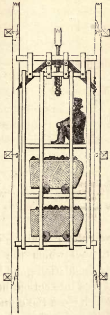
Fig. 32. Fontaine's parachute as it appeared at the colliery of Boussu, when the flat wire-rope broke with a weight of 2 tons.
