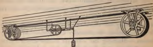
ROPE TRANSMISSION. "Wood System." With Take-Up.
