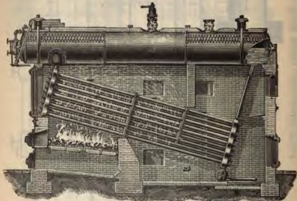
Babcock & Wilcox Boiler.
