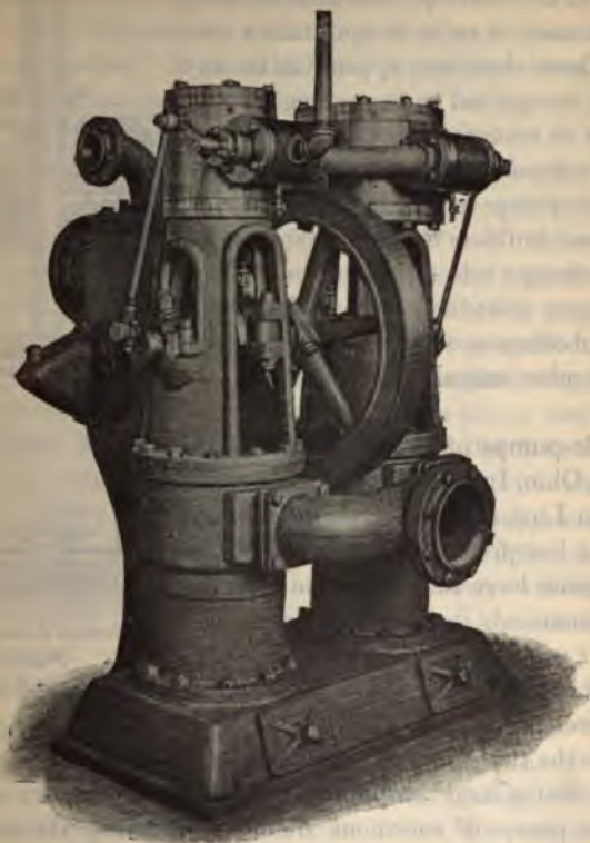
Barr Twin Pattern Vertical Air Pump and Condenser.
