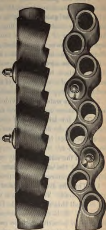
Headers of Babcock & Wilcox Boiler.
