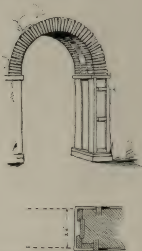
FIG. 2. ROMAN BRICKS AND SLAB CONSTRUCTION ARCHWAY AND PLAN OF ONE PIER. BRITFORD CHURCH
