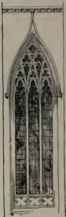
FIG. 54. TRACERY WITH TWO VARIETIES OF CUSPING. CHOIR, LICHFIELD. c. 1300
