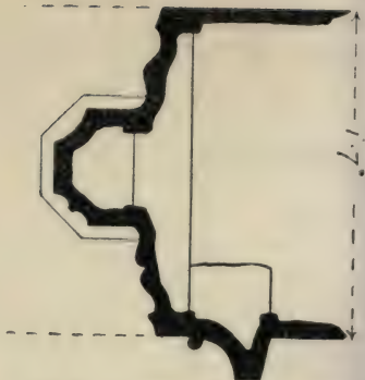
FIG. 82. SECTION OF DOORWAY
