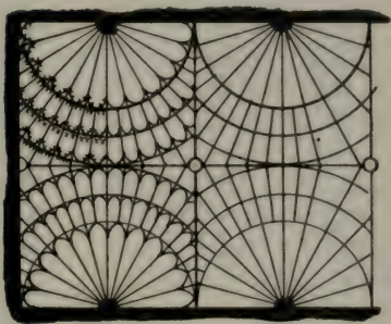
FIG. 88 PLAN OF FAN-VAULT, KING'S COLLEGE, CAMBRIDGE. 1512
