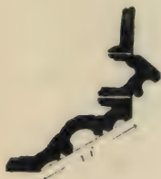
FIG. 80 SECTION OF DOORWAY
