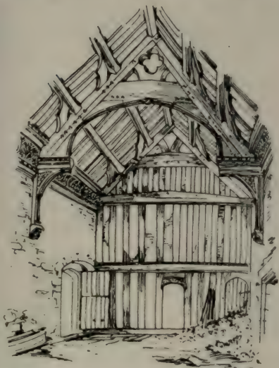
FIG. 89. HAMMER-BEAM ROOF, COCHWILLAN
