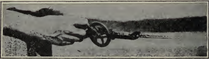
A hand-drill modified so as to wind up two rubber bands at once.
