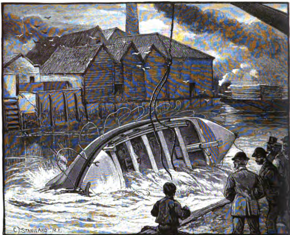
TESTING SELF-RIGHTING BOATS AT INSTITUTION'S YARD.
