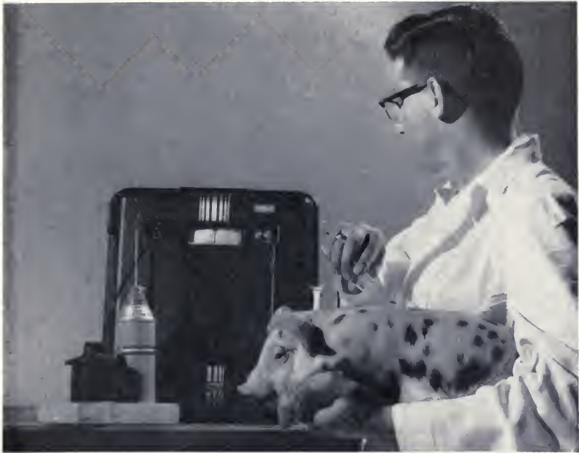
Measuring pig's skin temperature with touch thermocouple instrument.
