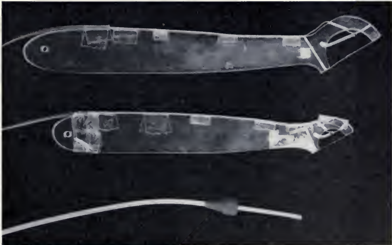
Thermocouple measuring instruments: (A) large plexiglass skin-temperature measuring instrument joining all seven strands of thermocouple wire; (B) small plexiglass skin-temperature measuring instrument joining only one strand of thermocouple wire; (C) rectal probe for measuring body temperature. (Fig. 10)
