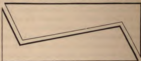
Fig. 59.—Diagram showing the mode of cutting out splints from a sheet of millboard.
