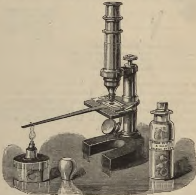
FIG. 15.—SIMPLE WARMING APPARATUS, COMPLETE, SHOWN IN OPERATION.
