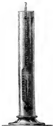
FIG. 39.—Urinometer floating in urine in a testing glass.
