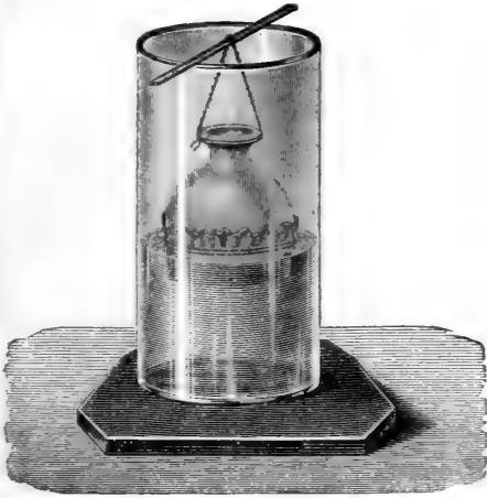
FIG. 7.—Dialyser. The lower opening of the bell jar suspended in water is tightly covered with parchment paper. The fluid to be dialysed is placed within this vessel ; the crystalloids pass out into the distilled water outside through the parchment paper.
