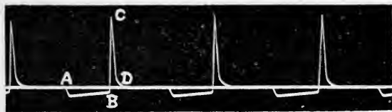
FIG. 14.—Graphic record of the secondary current from a well-designed coil.
