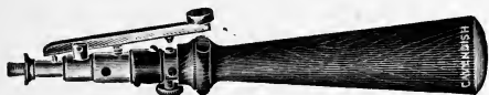
FIG. 43.—Testing Electrode. The chamois-leather-covered metal disc screws on the end. It is not shown in the figure.
