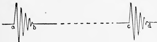
FIG. 46.—Intermittent Trains of Oscillations a to b—Train of oscillations, lasting \frac{1}{50,000} sec. b to c—Intermission, lasting \frac{1}{100} sec. c to d—Next train of oscillations
