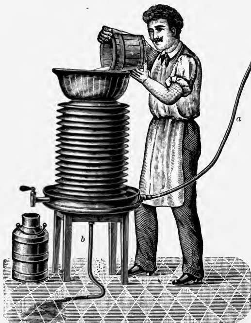
Schmidt's milk-cooler; a , entrance for cold water; b , exit for cold water.
