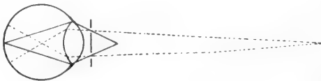
FIG. 56.—Scheiner's Experiment ——— represents rays from the near needle and - - - rays from the far needle.
