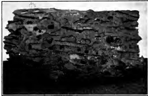
Piece of timber, showing holes bored by the shipworm.
