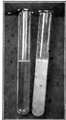
The limewater test; the tube at the right shows the effect of carbon dioxide.
