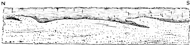
Fig. 3. New Reservoirs. Section towards S. end of Mitchley Marsh, seen July. 6th, 1900. Showing Clay, darkening towards the bottom, above gravel. Height of Section about 10ft., length about 50ft.
