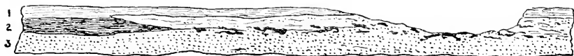
Fig. 5. New Reservoirs. 1. Surface Loam; 2. Peat; 3. Gravel and Sand. The irregular dark patches are fragments of the Stems of trees and plants, with other vegetable matter.
