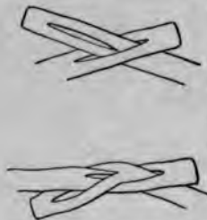
FIG. 302.—Double-slit splice for rawhide lines.
