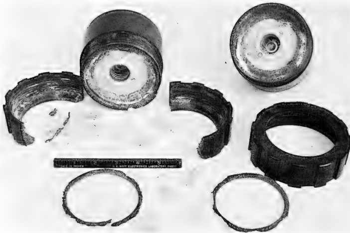
Figure 14. Components of two BUSHIPS lamp casings after testing to destruction.
