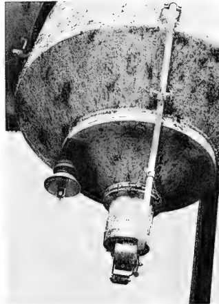
Figure 19. Edgerton lamp mounted on bathyscaph ballast tube for use with closed-circuit TV.
