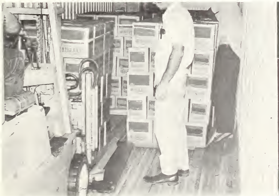
Figure 10.--Slipsheeted load of frozen food being pushed onto floor of trailer at processing plant.
