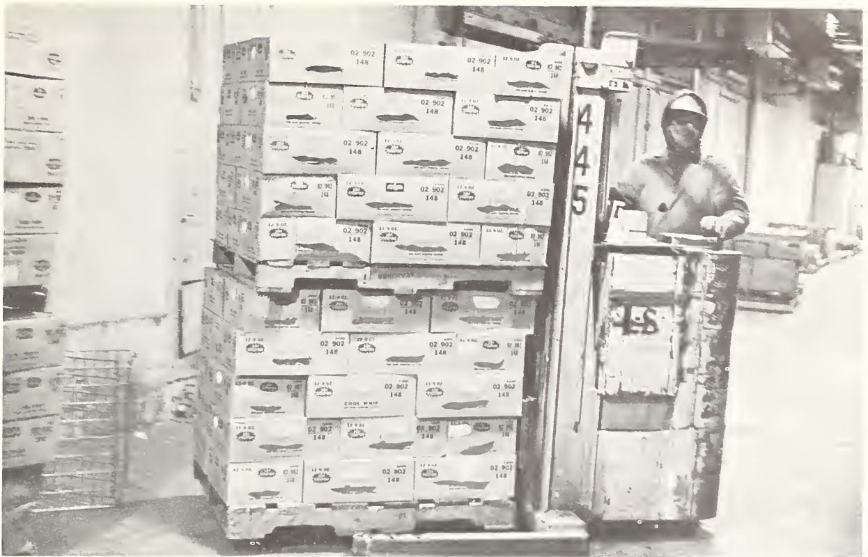
Figure 4.--Two pallet loads of frozen food being transported from loading dock by stand-up rider forklift truck to storage in warehouse.
