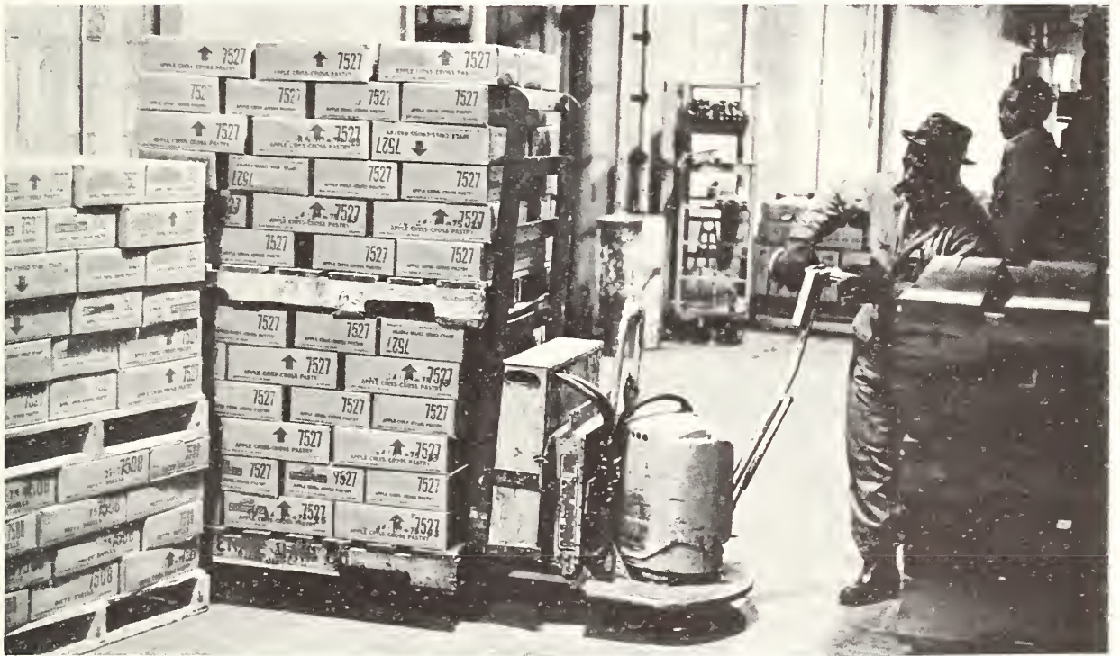
Figure 3.--Two pallet loads being removed from trailer as a single unit by electric pallet jack at wholesale warehouse.
