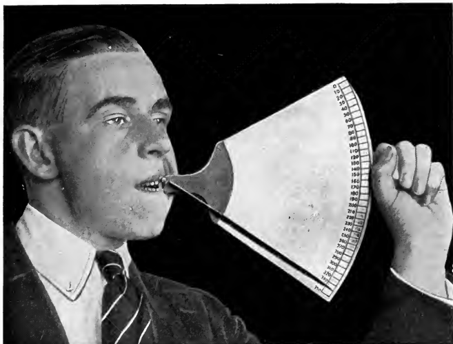
Fig. 39.—Gnathodynamometer. For measuring the force exerted by the closing of the jaws. This represents a man exerting a pressure equal to 340 pounds—over twice his weight.
