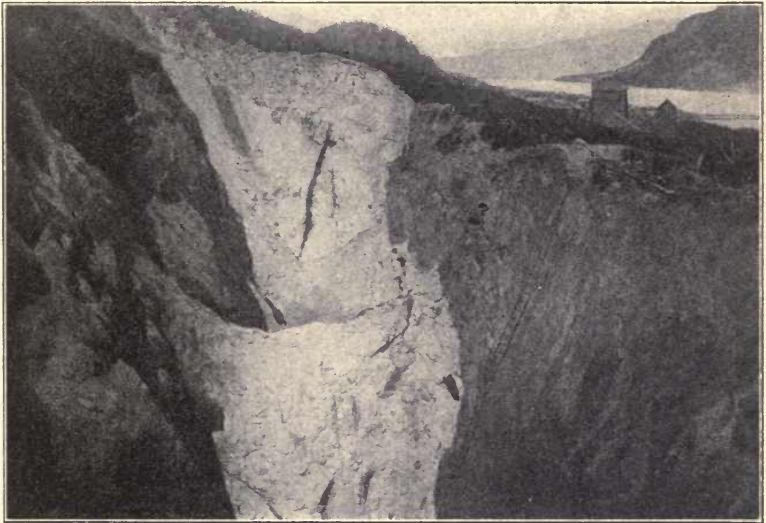
FIG. 21.—Open pit of the Treadwell mine, Douglas Island, Alaska, showing an albite-diorite dike that has been brecciated and impregnated with ore. After Spencer.
