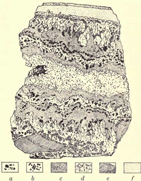
FIG. 45.—Specimen from the Pacific vein near Pinos Altos, New Mexico, showing crustification. a , Chalcopyrite; b , pyrite; c , zincblende; d , quartz; e , sericitized porphyry; f , carbonates, quartz, and iron oxide. After Paige.
