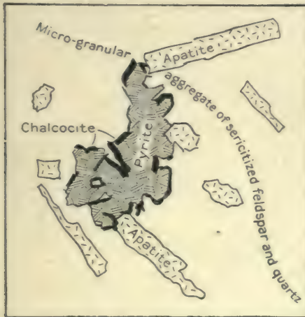
FIG. 73.—Group of pyrite crystals, showing secondary chalcocite along the edges. After Paige.
