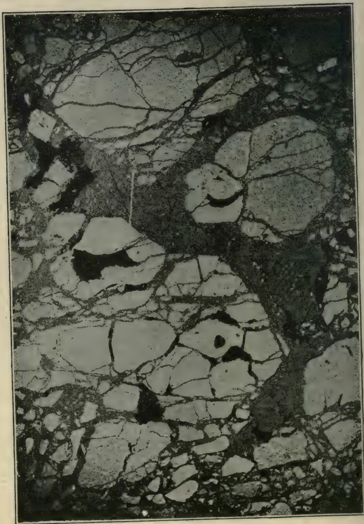
FIG. 72.—Photomicrograph of secondarily enriched ore from the lower part of the chalcocite zone, Morenci, Arizona, showing the occurrence of the later and richer sulphide through the pyrite. Dark gray = secondary chalcocite, developing by replacement in pyrite; light gray = pyrite; black = open field. After Lindgren,
