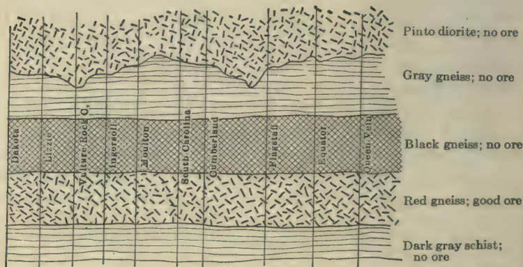
FIG. 67.—Diagram (plan) showing the rocks traversed by the Neihart veins and their ore content in the various rocks. After Weed.
