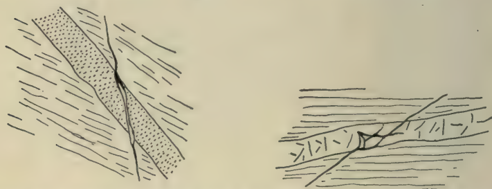
FIG. 66.—Sections showing the behavior of veins in passing through porphyry dikes, Cornwall, England; the values are segregated where the porphyry forms the walls of the veins. After De la Beche.
