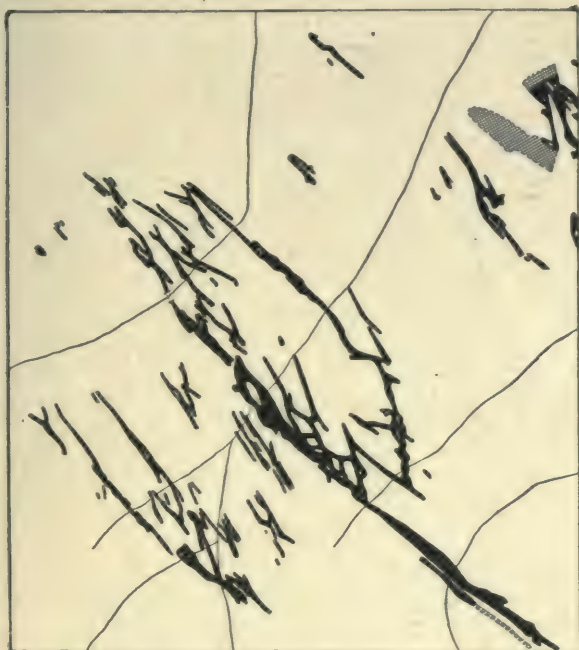
FIG. 32.—Map of the principal ore-shoots of the Bald Mountain area, Black Hills, South Dakota, showing the marked parallelism of the payable fissures. After Irving.
