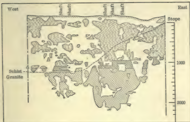
FIG. 65.—Section through the Dolcoath mine, Cornwall, showing the copper stopes where the vein is in schists, and the tin stopes where the vein traverses granite. After LeNeve Foster.
