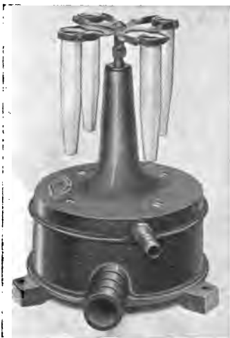
Fig. 33.—Ball-bearing water-motor centrifuge.
