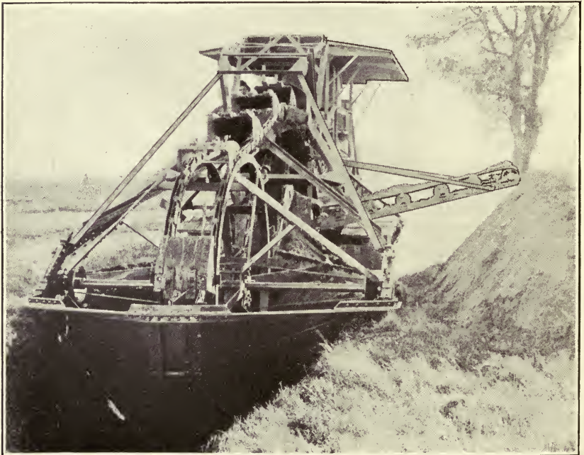
FIG. 2.—CONVERTIBLE TYPE OF WHEEL EXCAVATOR.
