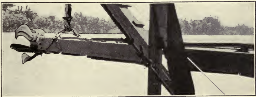
FIG. 3.—A TYPE OF CUTTER HEAD USED ON THE HYDRAULIC DREDGE.
