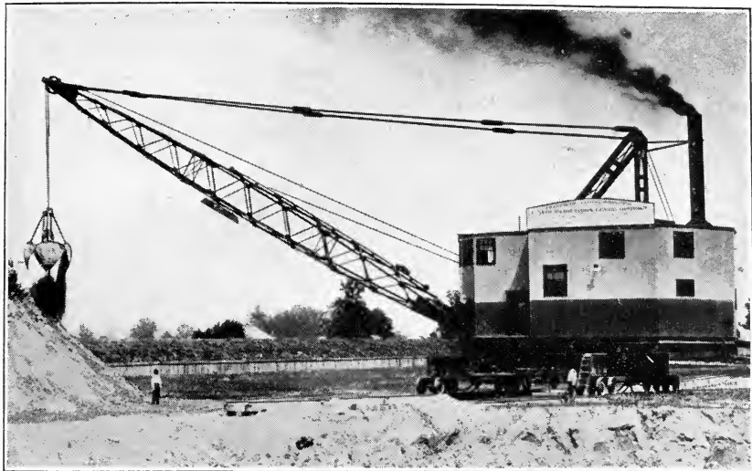
FIG. 1.—DRY-LAND ROTARY GRAB-BUCKET EXCAVATOR.
