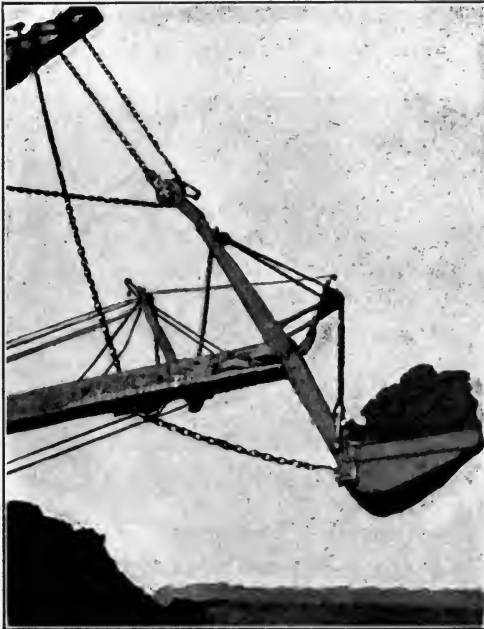
FIG. 39.—Dipper and dipper arm of walking dredge.
