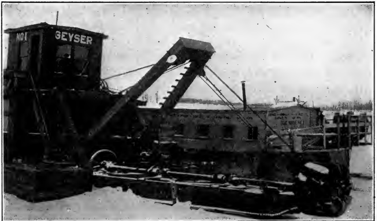
FIG. 115.—Cutter and suction pipe of hydraulic dredge. (Courtesy of N. Y. State Engineer.)
