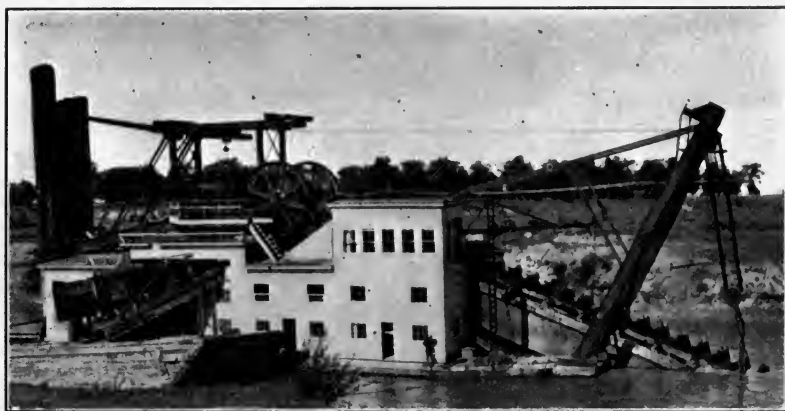
FIG. 107.—Ladder dredge provided with trough for discharging excavation into barges. (Courtesy of the Bucyrus Co.)
