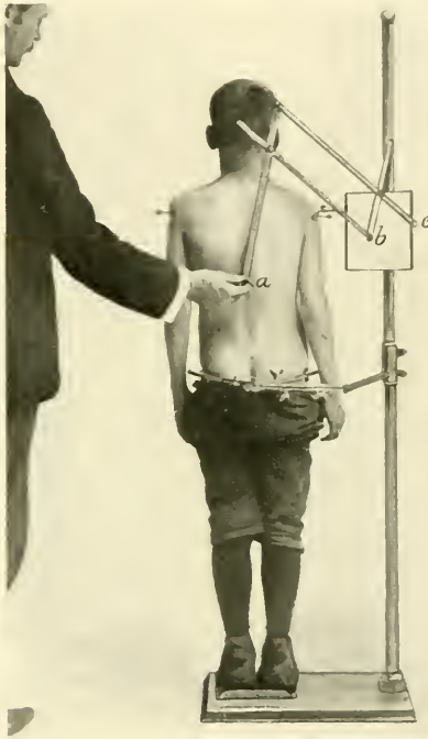
Fig. 241.—Making a tracing of the lateral deviation by the author's scoliosimeter: a , Pointer which follows the line of the spinous processes and tips of the scapulae; b , pencil recording the tracing on paper to the scale of 1 to 4; e , fixed point of the pantograph.
