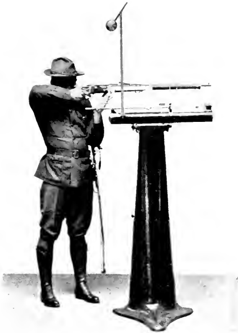
Fig. 127.—Subtarget gun machine for rifle practice in high schools (Handbook of Public School Athletic League, N. Y.).
